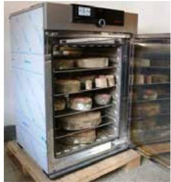
Figure 14: Drying of disc samples
